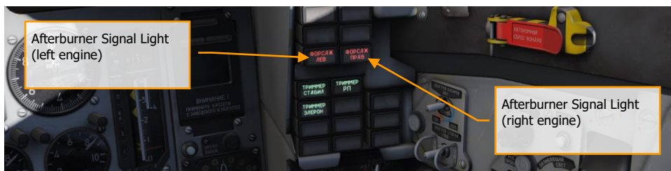
Figure 26: "Форсаж" (Afterburner) signal lights
