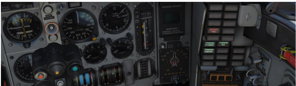
Figure 68: "Engine Start Left" signal lamp ("ЗАПУСК ЛЕВ")
