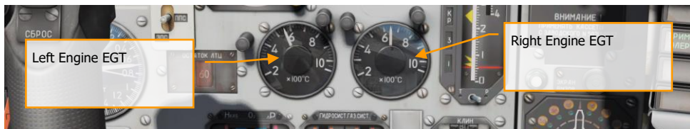
Figure 28: Interstage Turbine Temperature Indicators
