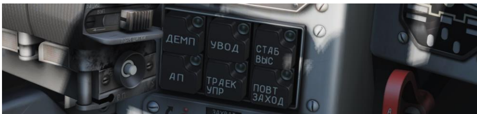
Figure 32 – AFCS push-light switches
