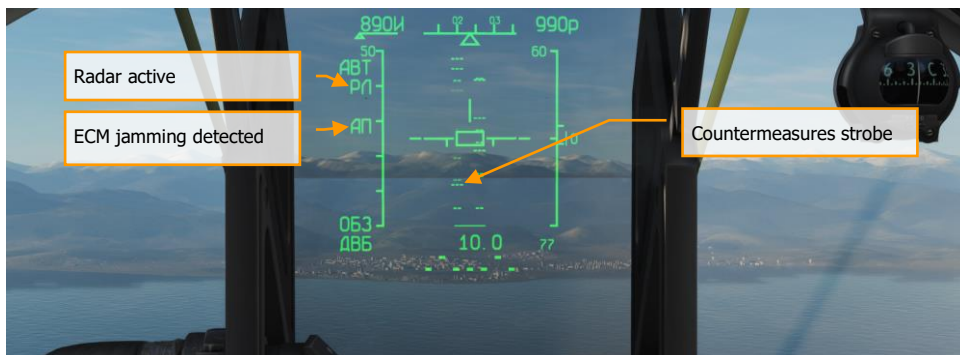
Figure 44: SCAN Mode with jammer strobe
